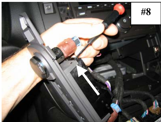
Using a small flat head screwdriver, unclip fastener
